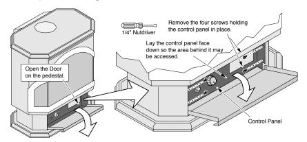
Access the firebox and remove the burner pan following the directions below
